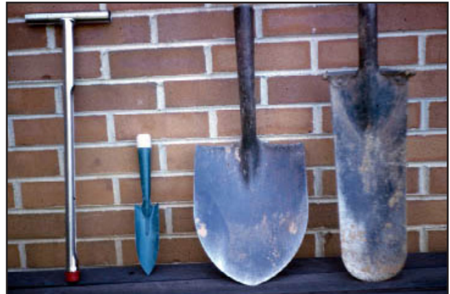
Figure 1. From left to right: a stainless steel soil probe, a hand garden trowel, shovel, and a spade. All acceptable tools for collecting a soil sample.
